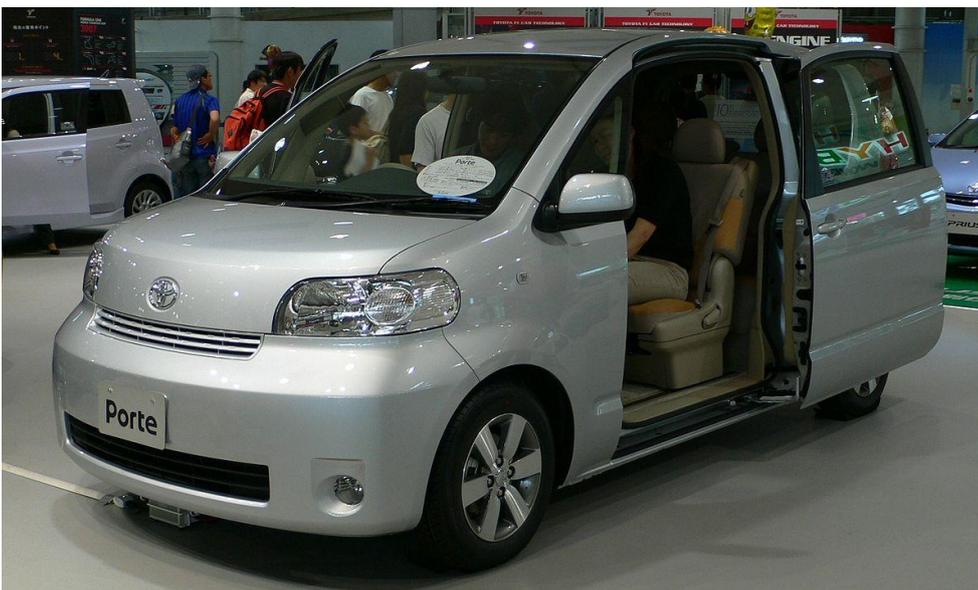
Fig. 2.37: Toyota Porte with an electric sliding front door on the passenger side ([upload.wikimedia.org/wikipedia/commons/thumb/7/7f/Toyota Porte\\_02.jpg/1200px-Toyota Porte\\_02.jpg](http://upload.wikimedia.org/wikipedia/commons/thumb/7/7f/Toyota_Porte_02.jpg/1200px-Toyota_Porte_02.jpg))
