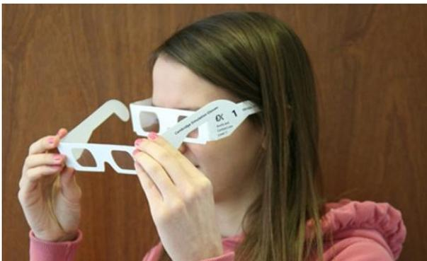
Fig. 2.21: Cambridge simulation glasses: Different levels of impairment are simulated by wearing different numbers of glasses.
